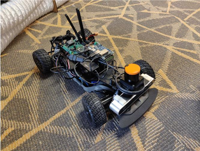
Fig. 1. Visualization of our experimental F1/10 hardware platform. This platform is a one-tenth scale RC car that has been altered to operate autonomously with the support of a sensor and compute architecture for autonomous decision-making [4].
