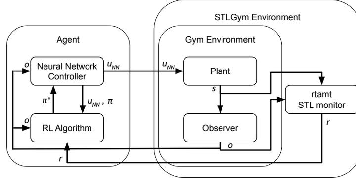
**Fig. 2.** A representation of how STL Gym wraps around the user’s environment to record signals and replace the reward function.
