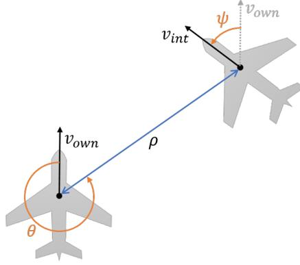
**Fig. 2 Diagram of the ACAS Xu physical variables.**
