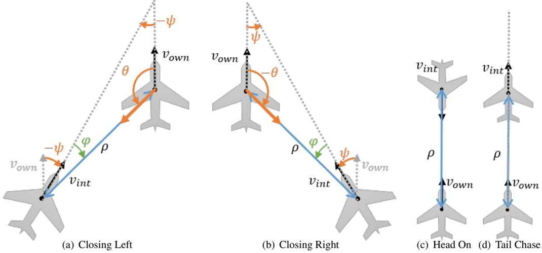
**Fig. 5 Closed Loop Test Case Geometry Examples**
