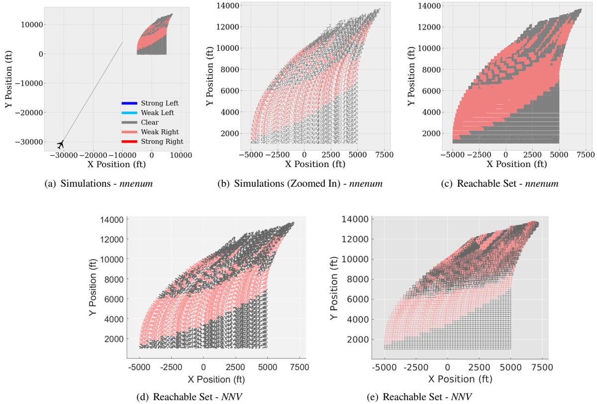
**Fig. 12 Left Gaining  $\varphi_{ACL}$  with initial ownship uncertainty  $x_0, y_0 = [\pm 5000, \pm 200]$ .**
