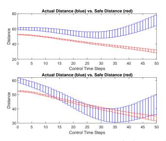
Fig. 3: Two scenarios of the ACC system. In the first (top) scenario  $(v_{lead}(0) \in [29, 30]m/s)$ , safety is guaranteed,  $D_{rel} \geq D_{safe}$ . In the second scenario (bottom)  $(v_{lead}(0) \in [24, 25]m/s)$ , safety is violated since  $D_{ref} < D_{safe}$  in some control steps.
