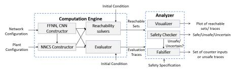
Fig. 1: An overview of NNV and its major modules and components.
